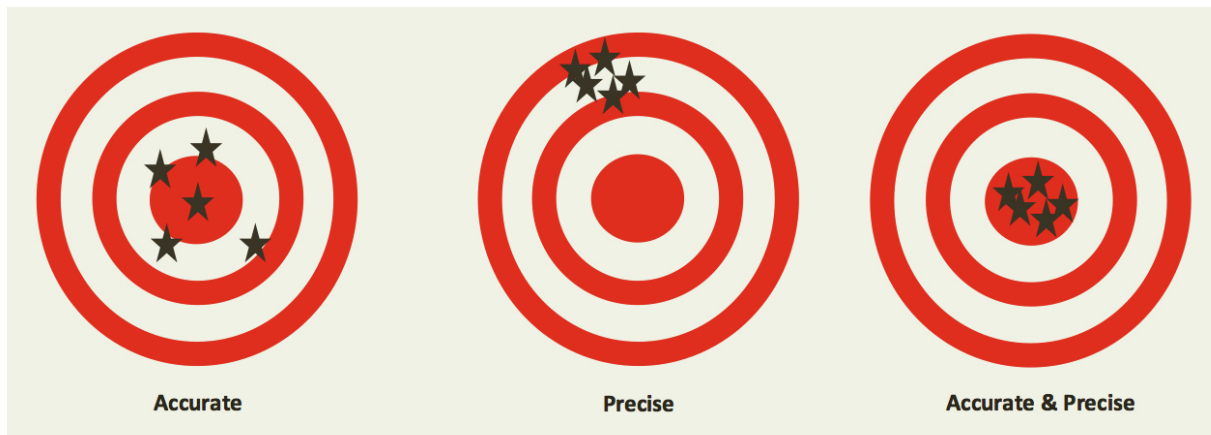
Figure 3 Schematic diagram explaining the difference between precision and accuracy
