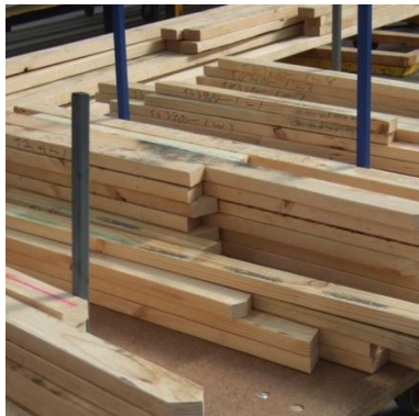
Figure 41: Pine truss chords
